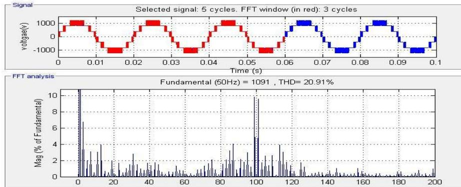
Fig. 7. THD analysis of cascaded H bridge topology
