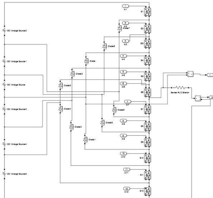
Fig 8. Simulink model of NPC MLI
