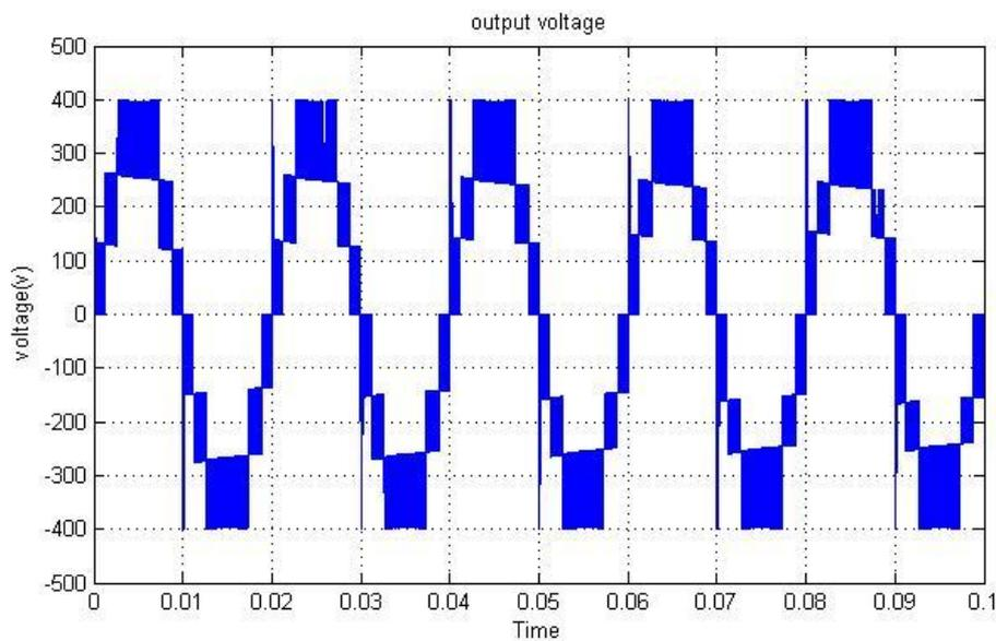
Fig. 9. Output voltage of new topology with seven levels
