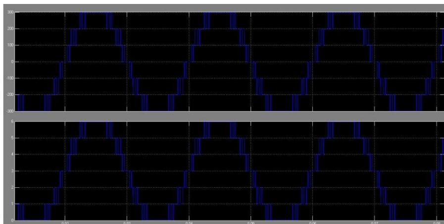
Fig 9. Output voltage waveform with seven levels for NPC MLI
