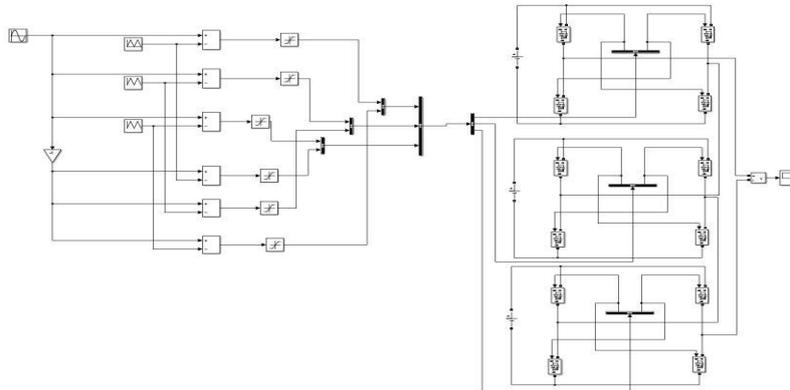
**Fig. 5.** Simulation model of cascaded multilevel topology
