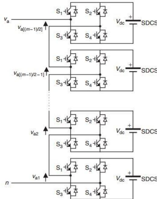
Fig. 1. Structure of a multilevel cascaded H-bridge inverter[2]
