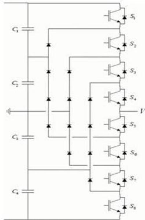
Fig. 2. Seven level diode clamped inverter[5]
