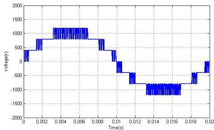
**Fig. 6.** Output voltage with seven levels of cascaded MLI
