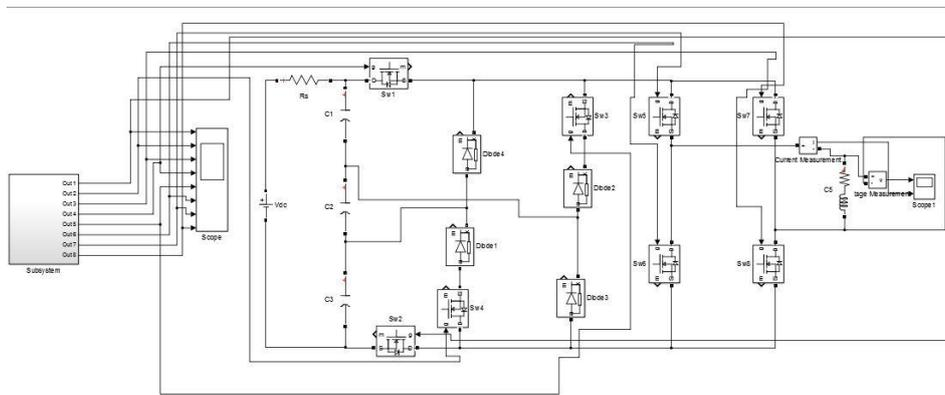
Fig. 8. Simulation model of new topology with less number of switches
